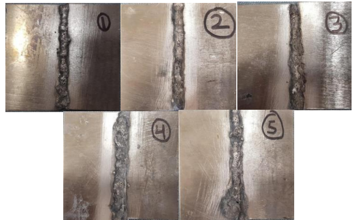
Figure 3.8: - Sample 1-5 In Decreasing Order of Welding Speed Keeping Welding Current and Voltage Constant
