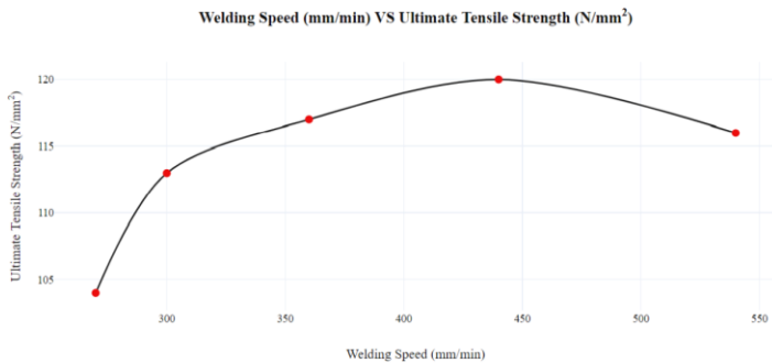
Figure 3.9: -Effect of Welding Speed on Ultimate Tensile Strength
